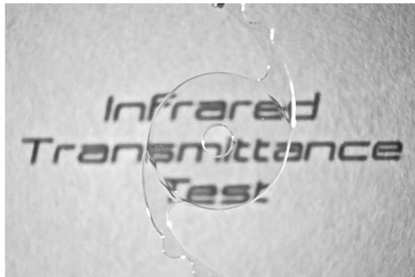
**Figure 3.** The black hydrophobic acrylic presents a window of transmission of IR light, enabling fundus examination with IR equipment.
