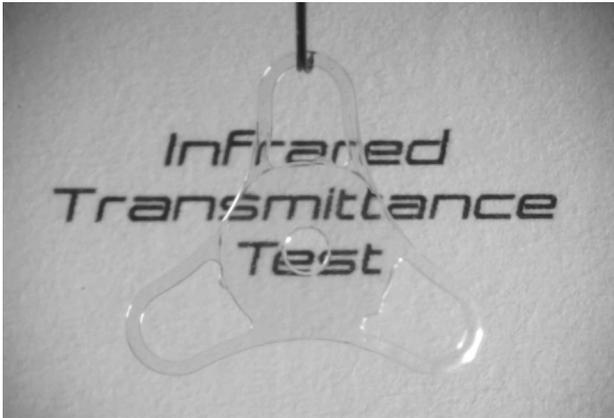
**Figure 6.** The implant is 100% transparent to IR light, allowing fundus imaging after implantation.
